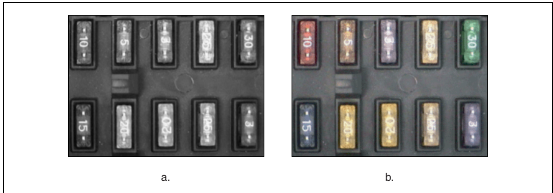
Figure 14-16. Benefit of Adding Color to Fuse Box Inspection
